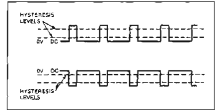
Figure 3. To enable a count on these waveforms the trigger level control must be out of PRESET to shift the hysteresis positive (upper waveform) or negative (lower waveform).
